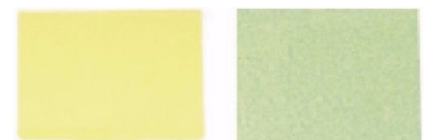
The new intensity labels 4001 begin as A bright yellow color (left). As they are exposed to UV they Become increasingly more green.
