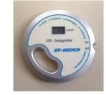
The UV-Integrator 140 is a high quality UV measuring instrument. It is used to measure UV energy of different light sources, especially on printing machines. It was specially designed with a recess in the housing for better handling. It is ideal to ensure quality control of printing and drying processes.
