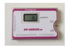
The UV-Integrator 151 is a high quality UV measuring instrument. It is used to measure UV energy of different light sources, especially on printing machines. It is ideal to ensure quality control of printing and drying processes. Small size, heavy duty pass-through Integrator with very small dimensions. It is reliable and simple to use.
