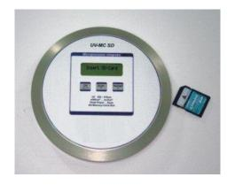
The UV-MC SD Microprocessor Integrator Low intensity is a self-contained, high quality UV measuring instrument. It is designed to measure, record and display peak UV intensity and UV dosage in the UV curing process.
