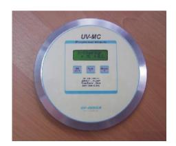
The UV-MC Microprocessor Integrator low intensity is a self-contained, high quality UV measuring instrument. It is designed to measure, record and display peak UV intensity, UV dosage and temperature in the UV curing process.
