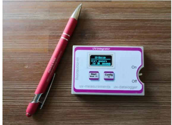
The UV Integrator 152 LED is a self-contained, high quality UV measuring instrument. It is designed to measure, record and display peak UV intensity, UV dosage and temperature in the UV curing process.
