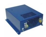
The EVG UV 20-42 AC is a fully electronic, adjustable AC ballast unit for UV-lamps from approx. 0.5 kW - 2 KW nominal power and specially designed for industrial use. It is specially tuned to operate with mercury discharge UV-lamps of 5-45 cm (2"-17") arc length. Dark phases during the zero axis known from standard, sinus shaped power supplies are eliminated by operating the lamps with a square-wave current.
