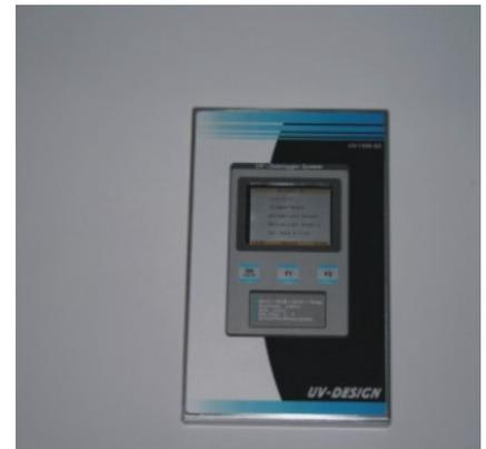
The **UV-1400 Colour RE Radiometer + Dosimeter** is a self-contained, high quality UV measuring instrument. It is designed to measure and record UV intensity and UV dosage in the UV curing process. Measuring results are indicated both, graphically and numerically on a big colour display.
